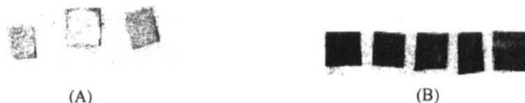
FIGURE 10 Test for the persistence of the activity of the immobilized anti-isoproturon antibodies on the plasma functionalized membranes. (A) Non sensitized membranes checked for the absence of non specific retention of the isoproturon enzyme conjugate. (B) Sensitized membranes incubated with isoproturon enzyme conjugate
